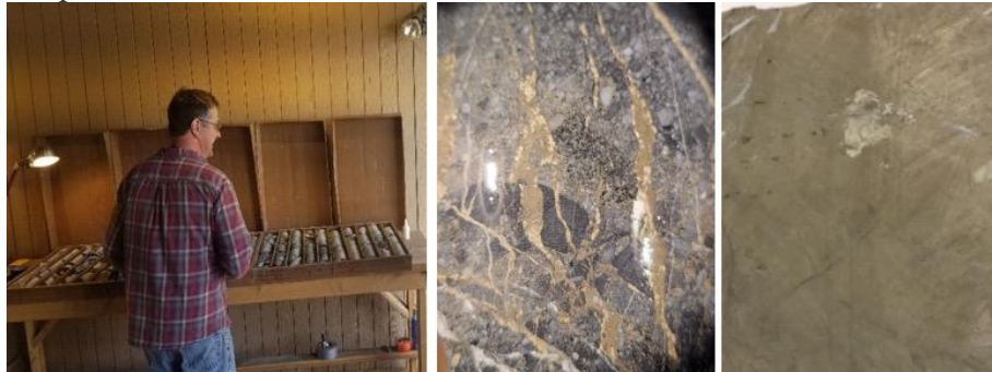
Drill core from Cooke Mountain project – highlighting new zone with veined and massive sulfides at Lamefoot South
