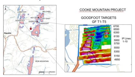
The Goodfoot survey was conducted over the entire property on 200 metre line spacings with 50 metre dipoles and N = 1 to 8 array in order to penetrate to approximately 225 metres. The data was subsequently
