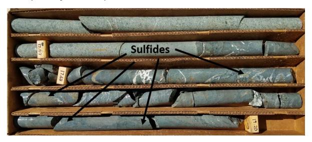
Photo: Box of core showing increasing sulfides in clastic rocks
