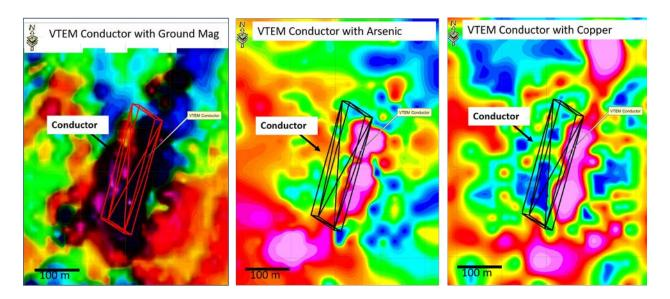
Figures show VTEM EM, ground magnetics and soil geochemistry associated with the SE-01 Target. Note the strong correlation between the various survey datasets making this a priority exploration target.
